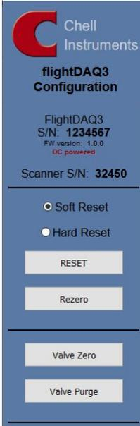
Figure 5.1 above shows the first page viewed when navigating to the webserver. The menu at the top allows the user to choose what is visible in the central window, and the sidebar (shown left) shows information and has a select few commands that are useful regardless of the central page the user is on. The function of the controls on the sidebar is detailed in the subsequent table (Table 5.1)
